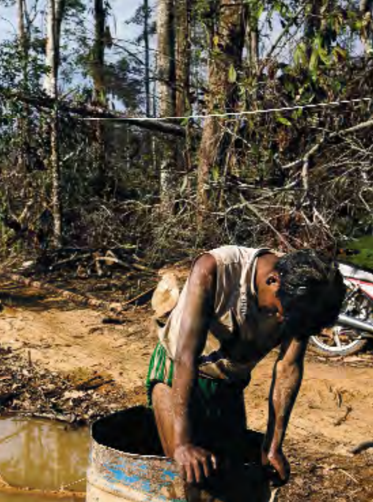
Near the mining camp of Lamal, a miner works poisonous liquid mercury into sludge with his bare feet; gold amalgam will form and be collected. Peruvian officials say 30 to 40 tons of mercury end up in Amazonian rivers each year.
