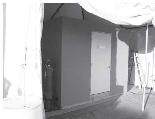
Figure 1. Photograph of the exterior view of test room and tent enclosure. Room dimension = 2.9 m long \times 3.5 m wide \times 2.0 m high. The door and window are located on the opposite sides of the shorter walls.
