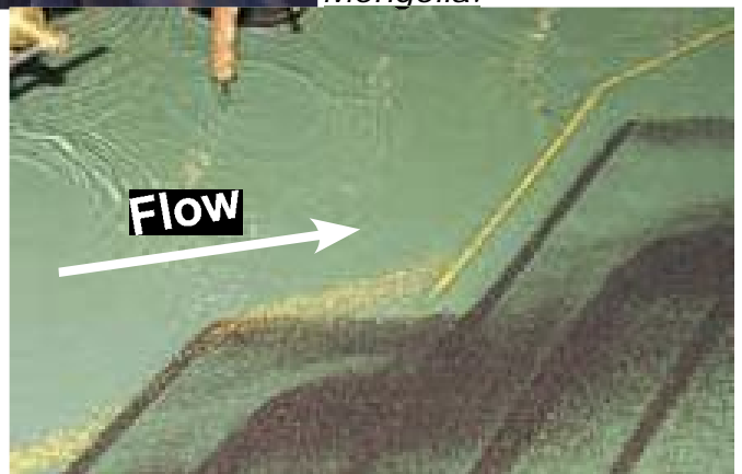
A large shaking table is used at a small-scale mercury free processing plant in Mongolia.
