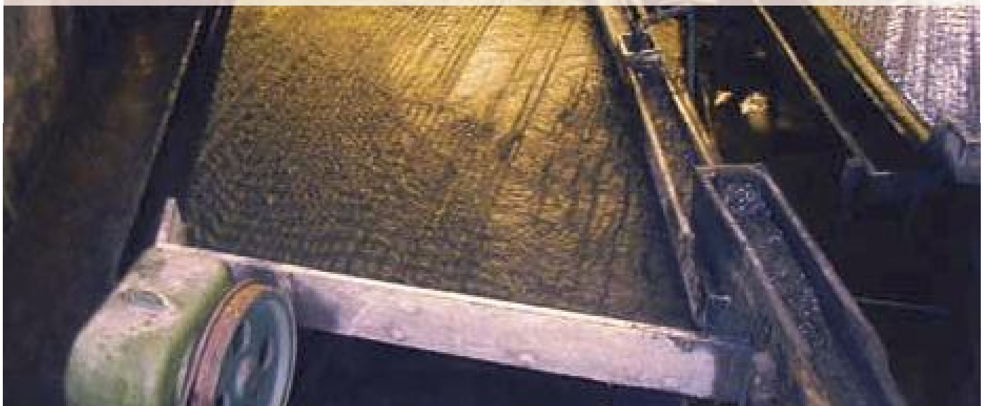
⑤ Sluice and mill concentrates both go to shaking table for secondary concentration.
