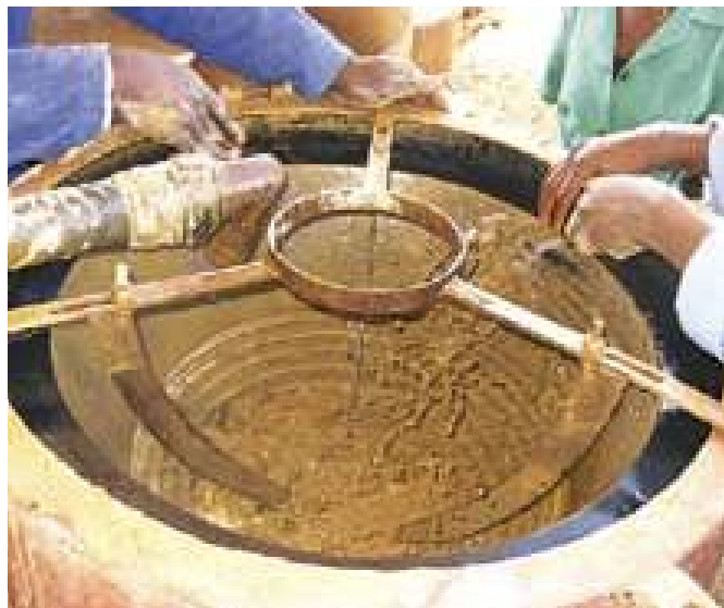
The Icon™ machine shown at left, made by Falcon Concentrators is designed to process up to 2 tonnes ore per hour. Models of this type range from 5-10 thousand $US. Below this small-scale centrifuge constructed in Zimbabwe uses turbulence bars which act to keep the concentrate bed active. This is not an efficient centrifuge but is relatively cheap at an approximate cost of 1-2 thousand $US.
