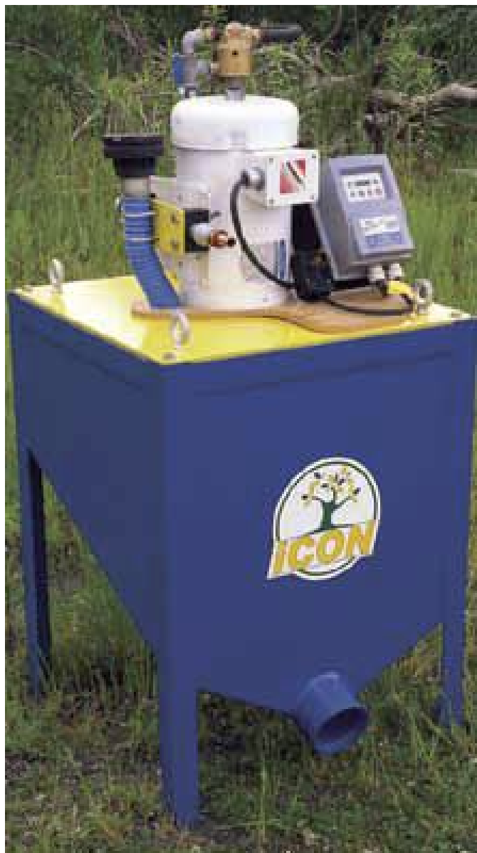
The Icon™ machine shown at left, made by Falcon Concentrators is designed to process up to 2 tonnes ore per hour. Models of this type range from 5-10 thousand $US. Below this small-scale centrifuge constructed in Zimbabwe uses turbulence bars which act to keep the concentrate bed active. This is not an efficient centrifuge but is relatively cheap at an approximate cost of 1-2 thousand $US.
